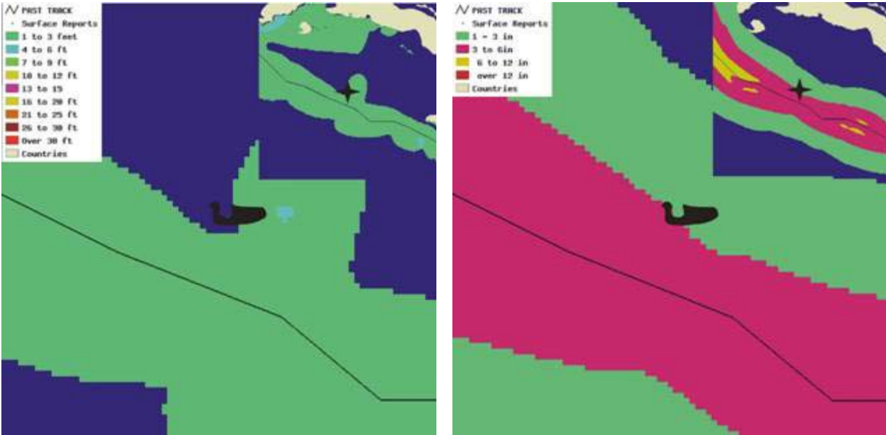
Figure 4.4 Storm surge height and accumulated rainfall estimation from TAOS model for Ivan.
